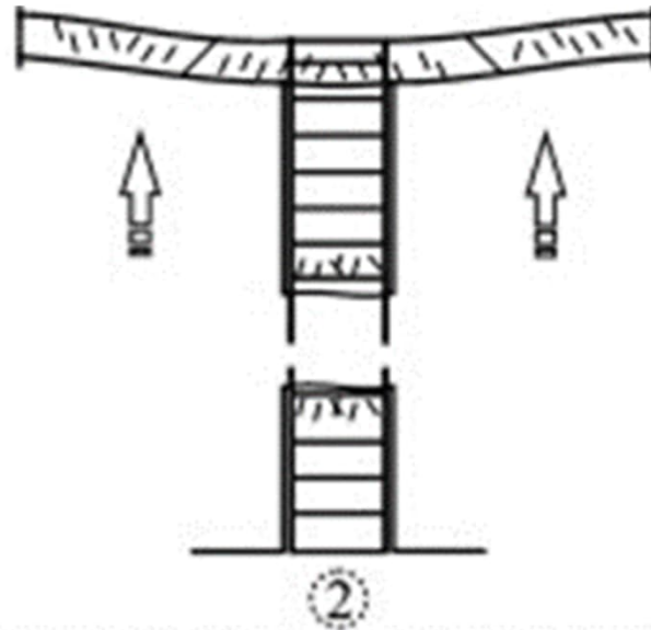
Fracture of column under the big axial tension caused by explosive pressure
