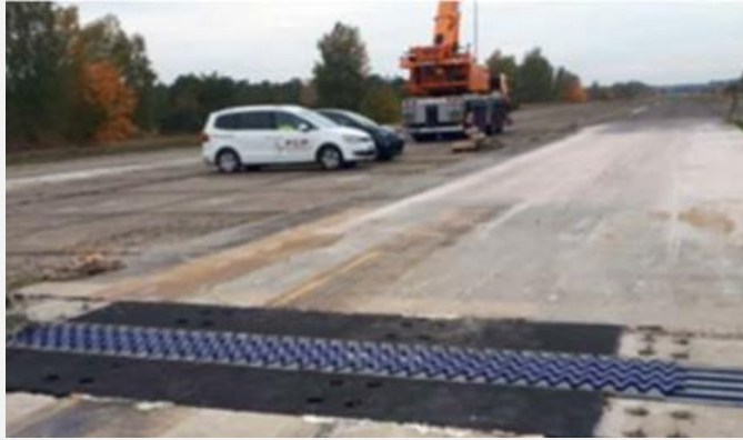
Specially constructed test specimen for noise testing of modular joint
